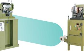
It can automatically cut, shape, seal, hammer Weld and assemble metal wire into chain.
